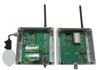
This *XTension* radios utilizes low power frequency hopping spread spectrum 900 MHz ISM radios. The base station is powered via the SDI-12 bus while the remote radios have internal user replaceable batteries.
